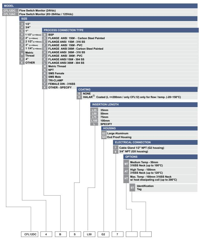
Max. insertion length for Halar coating is 200mm Insertion length over 100mm, process connection from 3/4" NPT/ BSP
